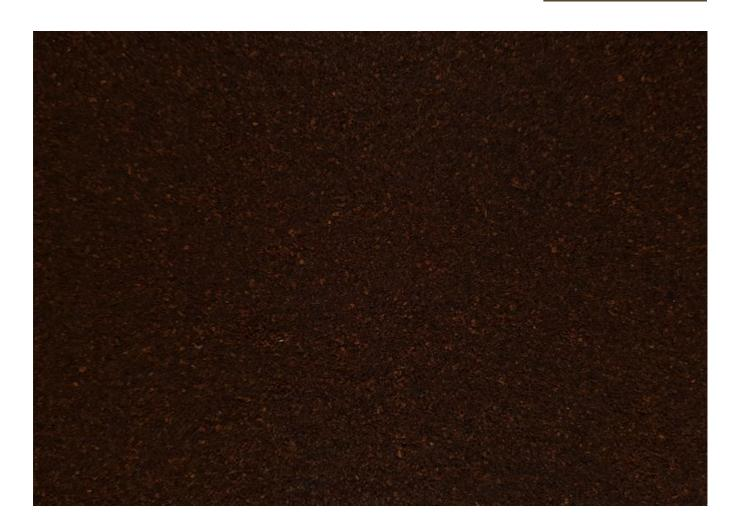
Vegan leather made from coffee powder, which can no longer be used as food and still exudes the typical stimulating coffee scent - on a thin flexible backing.
